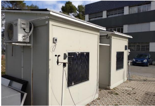
Figure 2: Testing cabins for BIPV windows and west view of the CIEMAT's BIPV ventilated façade.
